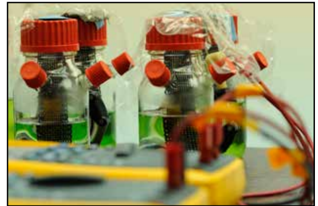
Microbial fuel cells contain different strains of bacteria and are monitored by multimeters at the Air Force Academy to determine the best environment for maximum energy output. Current research data shows the bacteria produces almost double the amount of energy during simulated hours of daylight vs non-daylight hours, making it a viable option for renewable energy through the process of photosynthesis. (U.S. Air National Guard photo/Staff Sgt. Michelle Y. Alvarez-Rea)
