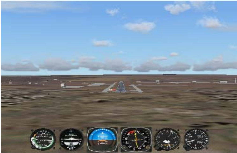
Figure 2. Simulated UAS display for landing task.
