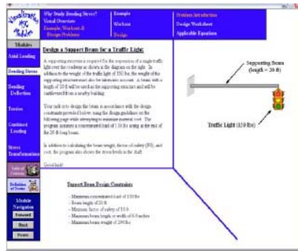
Figure 9: Traffic Light Beam Bending VisMOM
